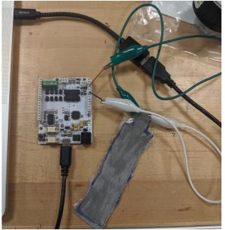
Double check your wiring and plug the Hapkit board back into the computer. Open the serial monitor (top right corner of Arduino program). You should be getting readings of the capacitance now (the length readings will not be accurate yet)
