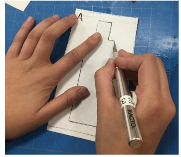
5. Laminate (completely cover) the cardstock and cardboard with tape and attach the cardstock to the cardboard (make sure to leave no gaps in the tape where the silicone can seep into). Wrap the tape through the hole you cut in the cardstock
