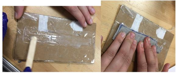
14.Carefully peel the sensor off the cardboard and flip it over, setting it back on the cardboard with the fabric you just attached face down.
