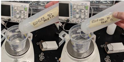
7. Mix the two parts together well using the mixing stick.
