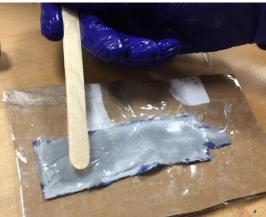
16. Press the fabric and silicone stack gently to push the silicone into the fabric.
