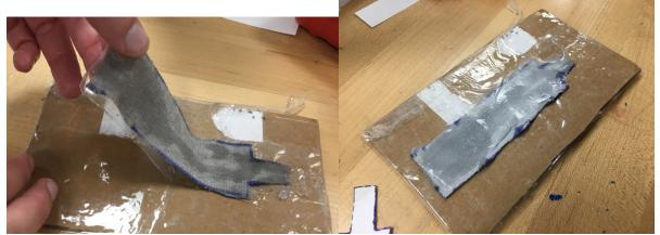
15.Using your mixing stick to spread a thin layer of newly mixed silicone on top of your set silicone. Take the second fabric piece and press it into the center of the silicone (again make sure the "shiny" side of the fabric faces outward)
