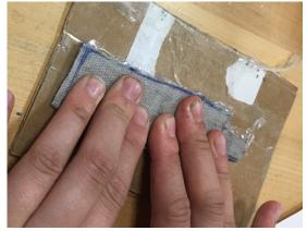
17. Return the soft sensor to the oven for another 20 minutes of curing
