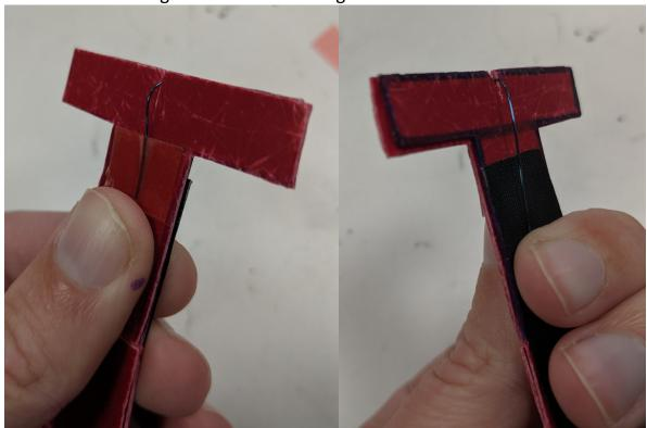
10. Pull the other end of the SMA wire through the second slit. The SMA should be on the same side as the fabric. Adjust the length so that the wire is taut when the joint is flat, and then tape down the end of the SMA wire.
