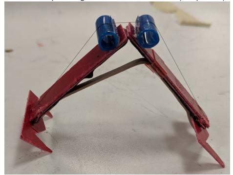
13. Repeatedly turn the battery pack on and off quickly to cause the robot to crawl (leaving the power on too long will cause the SMA wire to smoke). Try placing the crawler on different materials to see how is moves.
