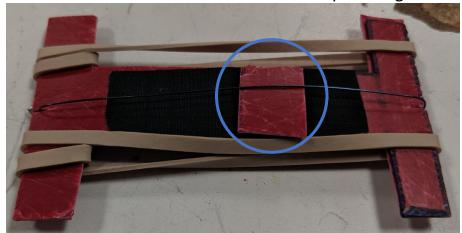
f. The robot is triggering but not jumping/not jumping high enough → Add rubber bands to create more stored energy or wrap rubber bands tighter to get a larger preload force
